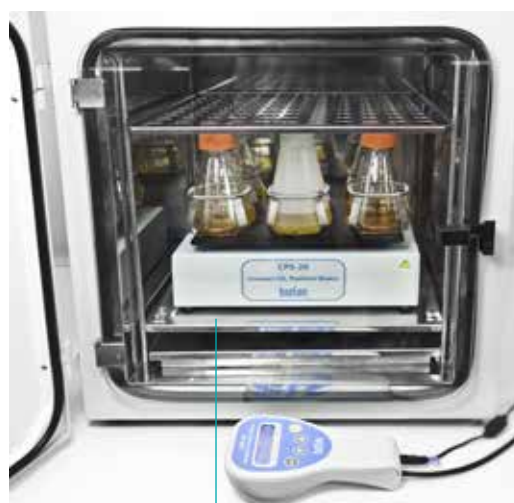
RS2, rack for CPS-20 installation
