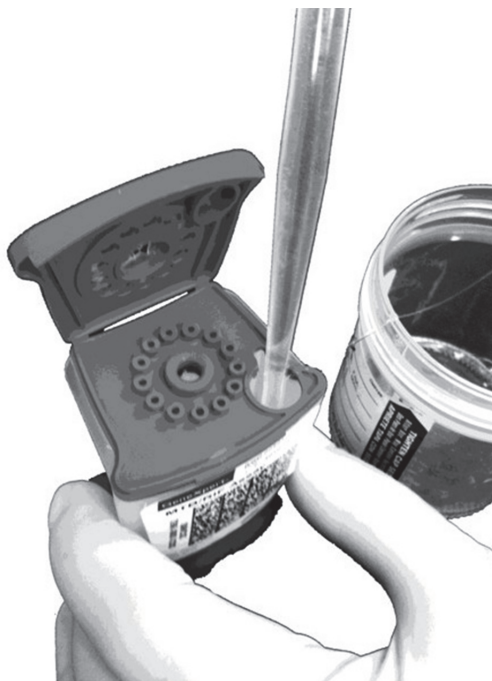
Figure 5. Dispensing Decontaminated Liquefied Sample into the Sample Chamber of the Cartridge
