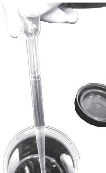
Figure 4. Aspirating to the Line on the Pipette
