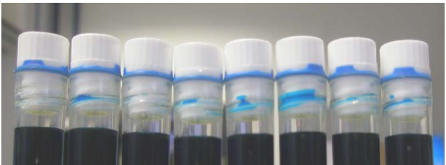
Fig. 4: High risk of carryover – unfavorable sample distribution – when using tubes with internal threading
