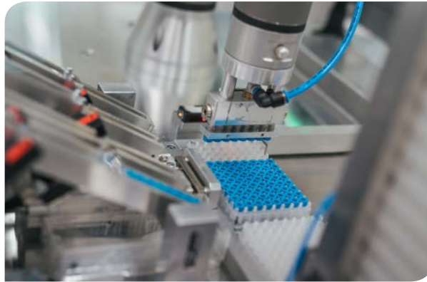
Automated Pick & Place for Cap Racking
