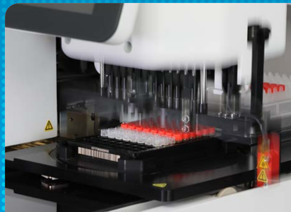
Fully-automatic 12 Channel Capper / Decapper
